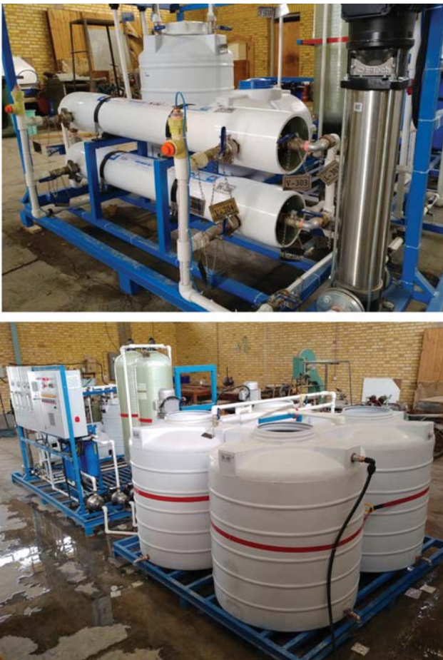
Fig. 5. The RO pilot plant at Hydraulic Lab of Shahid Chamran University of Ahvaz.
